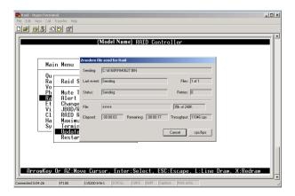
7. When the Firmware completes downloading, the confirmation screen appears. Press **Yes** to start program the flash ROM.
