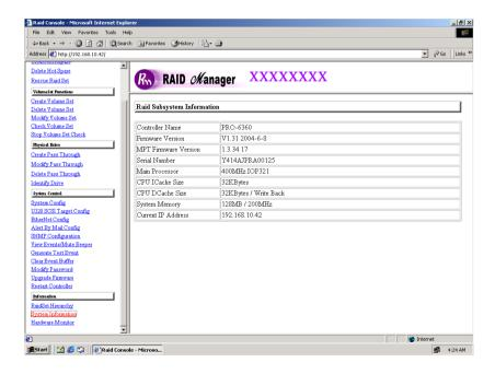
Use this feature to view the raid subsystem controller's information. The controller name, firmware version, serial number, main processor, CPU data/Instruction cache size and system memory size/speed appear in this screen.
