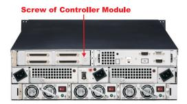
2. Unscrew and take off the cover of controller Module.
