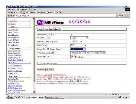
The number of physical drives in the raid subsystem determines the RAID levels that can be implemented with the raid set. You can create a raid set associated with exactly one volume set. The user can change the raid level, capacity, Volume Initialization Mode and stripe size. A hot spare option is also created depending upon the existing configuration.
