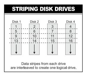
By striping the drives in the array with stripes large enough so that each record falls entirely within one stripe, most records can be evenly distributed across all drives. This keeps all drives in the array busy during heavy load situations. This situation allows all drives to work concurrently on different I/O operations, and thus maximize the number of simultaneous I/O operations that can be performed by the array.
