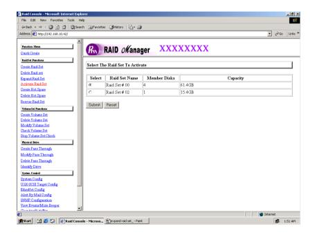
Click on the **Submit** button in the screen to activate the raid set that has removed one of disk drive in the power off state. The RAID subsystem will continue to work in degraded mode.
