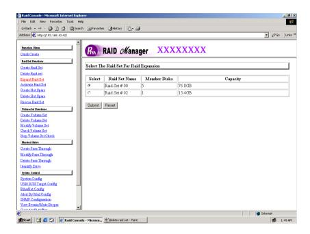
To expand a raid set, click on the **Expand Raid Set** link. Select the target raid set, which you want to expand it.
