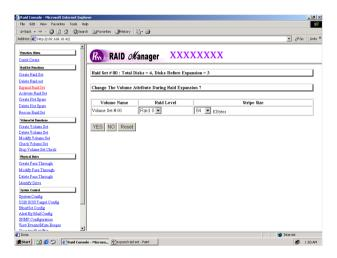
Migrating occurs when a disk is added to a raid set. Migration status is displayed in the raid status area of the Raid Set information when a disk is added to a raid set. Migrating status is also displayed in the associated volume status area of the volume set Information when a disk is added to a raid set.
