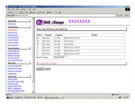
To create a raid set, click on the **Create Raid Set** link. A "Select The IDE Drive For RAID Set" screen is displayed showing the IDE drive connected to the current controller. Click on the selected physical drives with the current raid set. Enter 1 to 15 alphanumeric characters to define a unique identifier for a raid set. The default raid set name will always appear as Raid Set. #.
