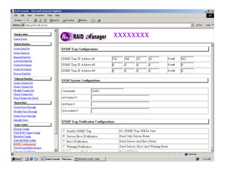
**SNMP Trap Configurations:** Type the SNMP Trap IP Address. The Port default is 162.
