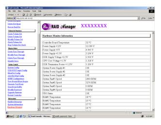
The Hardware Monitor Information provides the temperature, fan speed (chassis fan) and voltage of the internal RAID subsystem. All items are also unchangeable. The warning messages will indicate through the LCD, LED and alarm buzzer.
